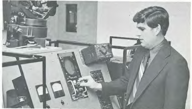
SEVERE WEATHER WITHIN a 100-mile radius of Manhattan will soon be detected on the screen of this radar set designed in the early 1950s for forward surveillance on a Boeing B52. Dr. Donald R. Hummels—judged the top educator in electrical engineering last year by students in that department—is making minor repairs on the radar set and recently was successful in obtaining an FCC license for its operation.
