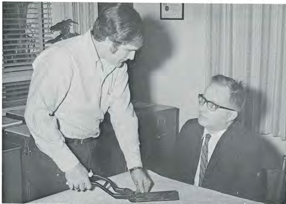
BIOMECHANIC TINSNIPS CUT DOWN FATIGUE —A pair of biomechanic tinsnips invented by Phillip B. Plant (left), senior in industrial engineering at KSU, reopen automatically when cutting heavy material. This saves on hand and finger muscle fatigue, says Dr. Stephan A. Konz (right), K-State industrial engineering professor. Konz says hand and finger muscles are not designed to reopen tinsnips and scissors when cutting through heavy material such as thick sheet metal.
