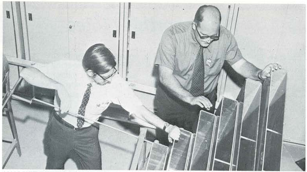
ANALYZE REACTOR SHIELDING — KSU researchers, Dr. Walter Meyer (l.) and James W. Thiesing, are analyzing the designs of various types of shielding used to protect workers and equipment working in and around nuclear power reactors. They are shown adjusting the geometry of water-filled aluminum cans taking place prior to measuring the intensity and spectrum of neutrons penetrating through water. Water is typically used as shielding around the cores of power and research reactors such as the KSU TRIGA Mark II teaching-research reactor.
