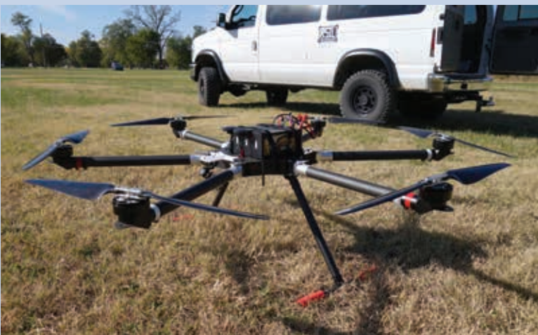
A U.S.-MANUFACTURED, LARGE MULTI-ROTOR UAS WITH A 22-POUND PAYLOAD CAPACITY
