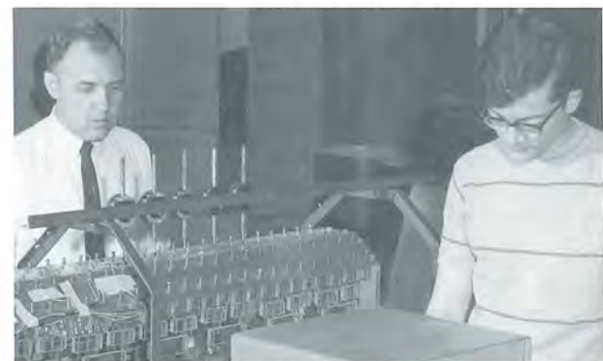
Swartz, left, circa 1969, works with student Warren Rosebraugh testing a model of a folded plate shell.
