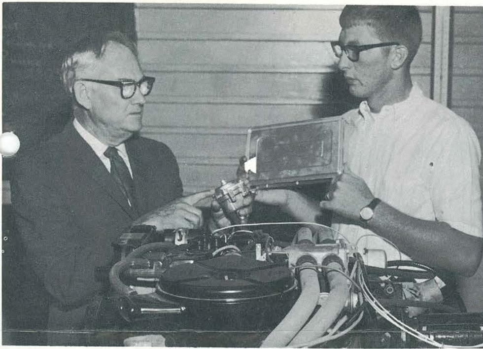
COMPUTERIZED FUEL INJECTION —Alley H. Duncan (l.), K-State professor of mechanical engineering, shows Bruce L. Wilson, senior from Abilene, Kan., a Volkswagen engine's computerized fuel injection system. This $850 engine, controlled by integrated computer circuits, is being used for teaching. The engine was donated to the KSU department of mechanical engineering through the Manhattan VW dealer, Larry K. Allingham. This semester a class taught by Dr. Ralph O. Turnquist, associate professor, will study the automatic control features of the engine.
